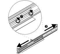
Remove the two screws **0** that hold the rails together so that the rails can slide outward **2**. Do not detach the rails.
