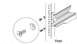
Align the bottom hole on the mounting rail with the bottom hole in the U-space (marked in step 3 above). Use the flat, Phillips head screws (10-32) and conical washers to attach the front rail to the rack. Position the rails so that the lip of the rail is on the bottom.
