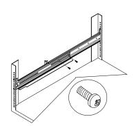
Expand the rails so that it spans from the front rack post to the back rack post. Replace the two screws (removed in step 1) that hold the rail sections together.
