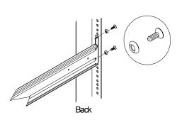
Attach the rail to the back rack post using the same hardware (10-32 flat head screws and conical washers) used in step 2. Repeat the process for the other rails.
