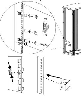
Install the Mounting Rails in the Rack
