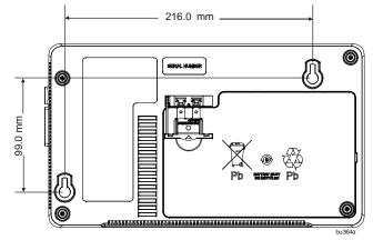
• Allow 5/16" (8 mm), of the screw to protrude from the wall.
